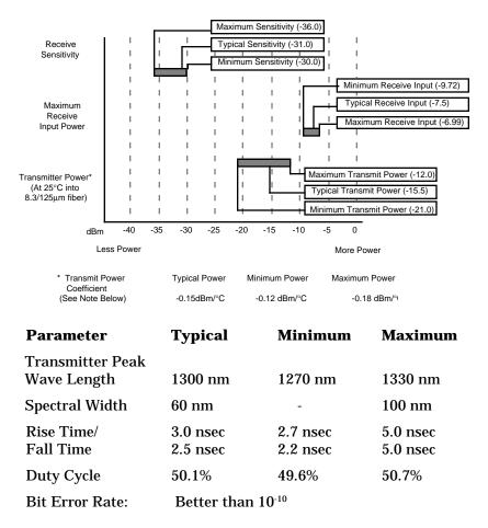
**Note**: The transmitter power levels given above are Peak Power Levels after optical overshoot. You must use a Peak Power Meter to correctly compare the values given above to those measured on any particular port. If you are measuring power levels with an Average Power Meter, add 3 dBm to the average power measurement to correctly compare the average power values measured to the values listed above (i.e. -33.5 dBm average + 3 dB = -30.5 dBm peak).
